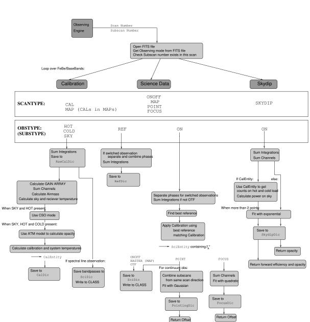
Figure 1: Sequence used for calibration of heterodyne data.
