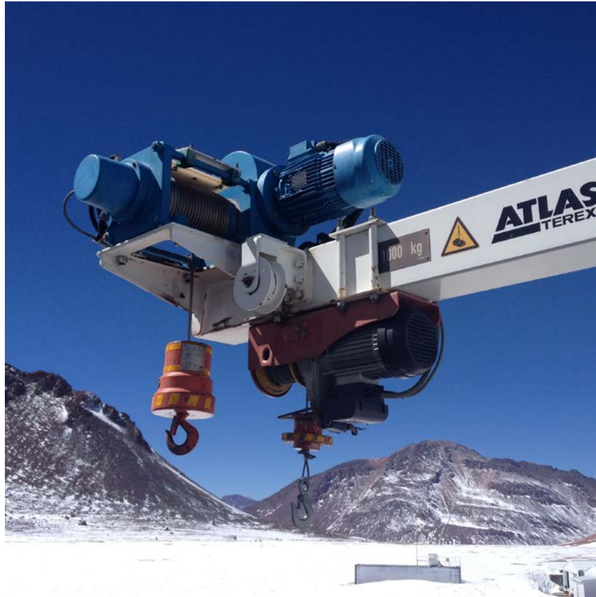
The crane located on the instrument platform of the telescope
